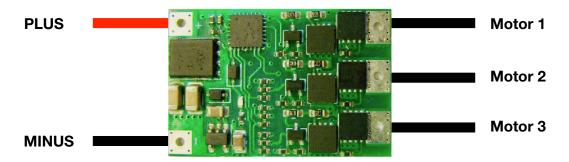
Scope of delivery: X89 Motor Controller for Brushless Motors
